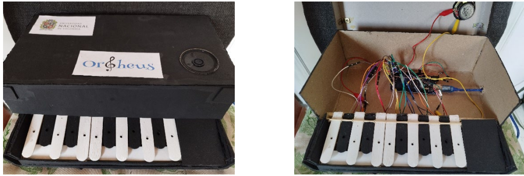
Figure 4. Musical keyboard (mini piano) of a single octave built for interaction with the software described in this paper.
