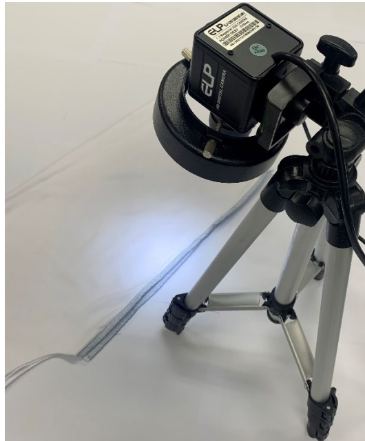
Figure 2. The setup for collecting images for the proposed dataset.
