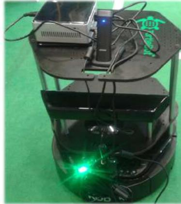
Figure 1: Turtlebot 2: Robotic Platform used for experiments with Kinect and WiFi devices.
